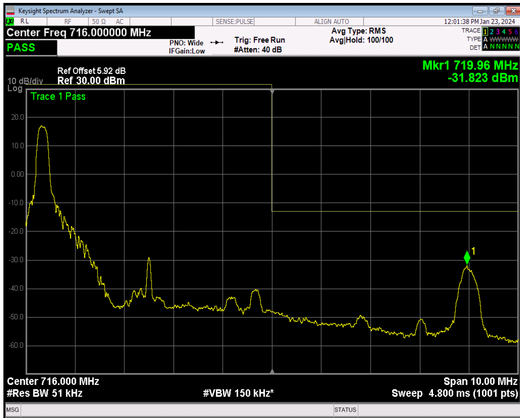
Band17 QPSK BW=5MHz Channel=23825 RB Size=1 Position=#Max
