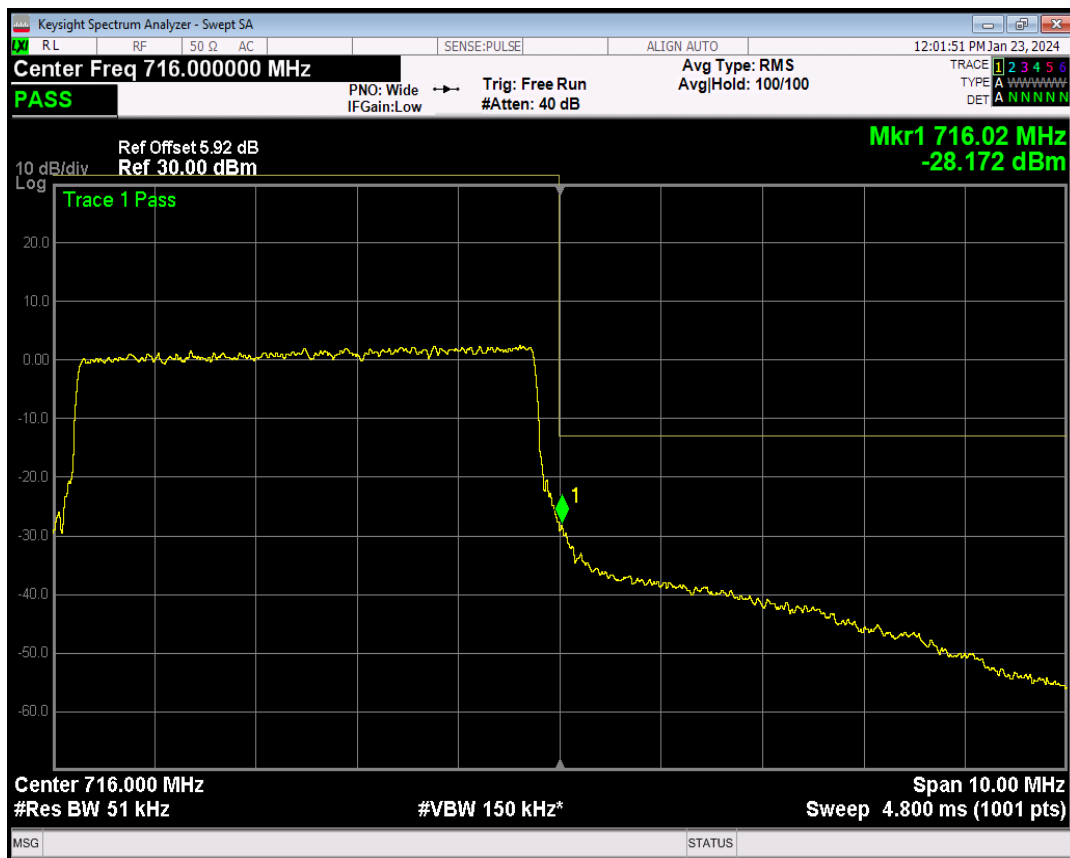
Band17 QPSK BW=10MHz Channel=23780 RB Size=1 Position=#0
