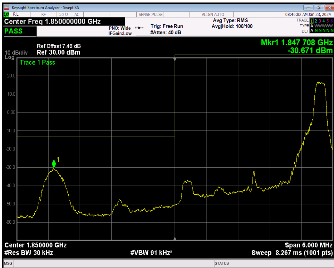
Band2 QPSK BW=3MHz Channel=18615 RB Size=15 Position=#0
