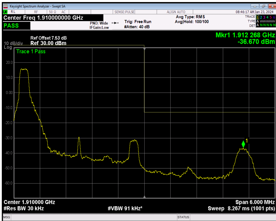
Band2 QPSK BW=3MHz Channel=19185 RB Size=15 Position=#0
