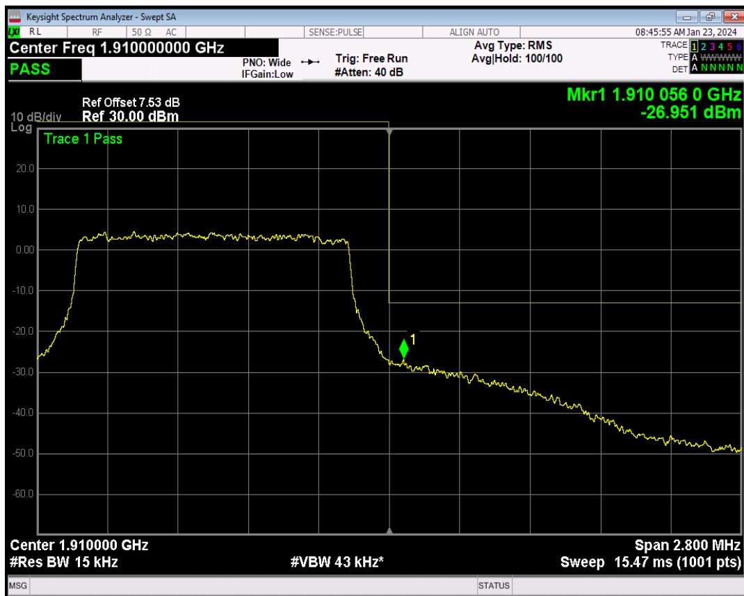
Band2 QPSK BW=3MHz Channel=18615 RB Size=1 Position=#0
