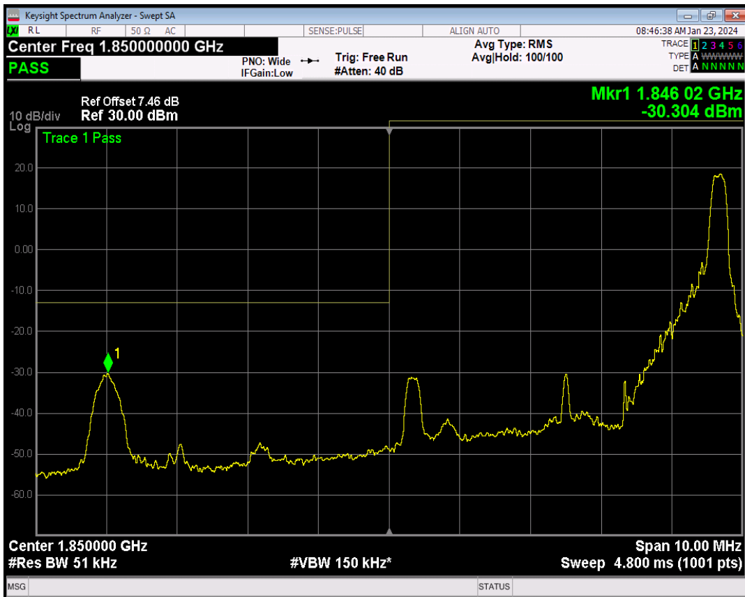
Band2 QPSK BW=5MHz Channel=18625 RB Size=25 Position=#0
