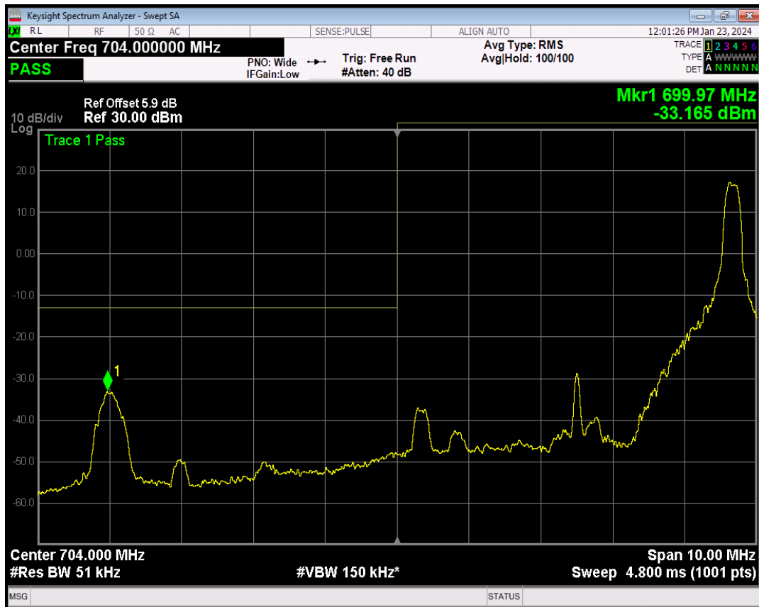
Band17 QPSK BW=5MHz Channel=23755 RB Size=25 Position=#0
