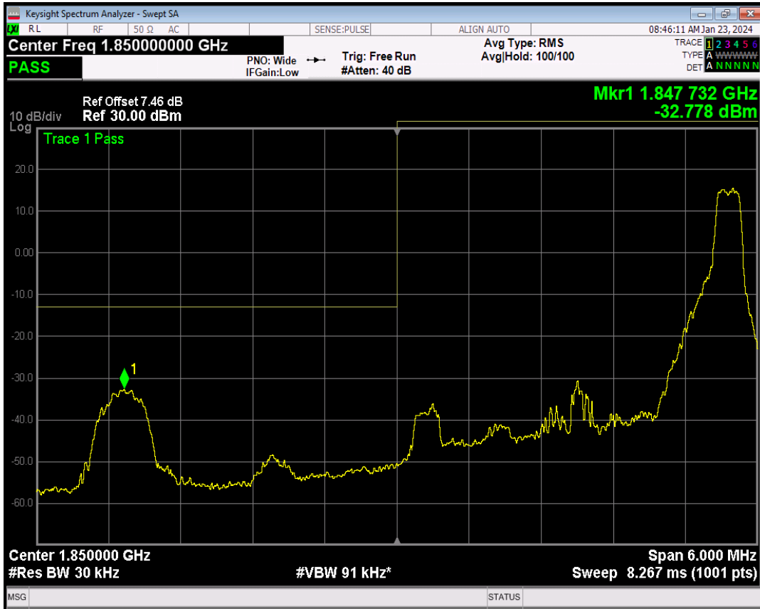
Band2 16QAM BW=3MHz Channel=18615 RB Size=15 Position=#0
