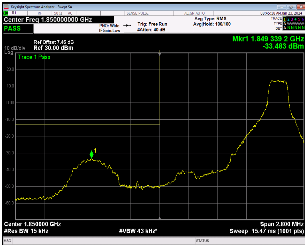
Band2 QPSK BW=1.4MHz Channel=18607 RB Size=6 Position=#0
