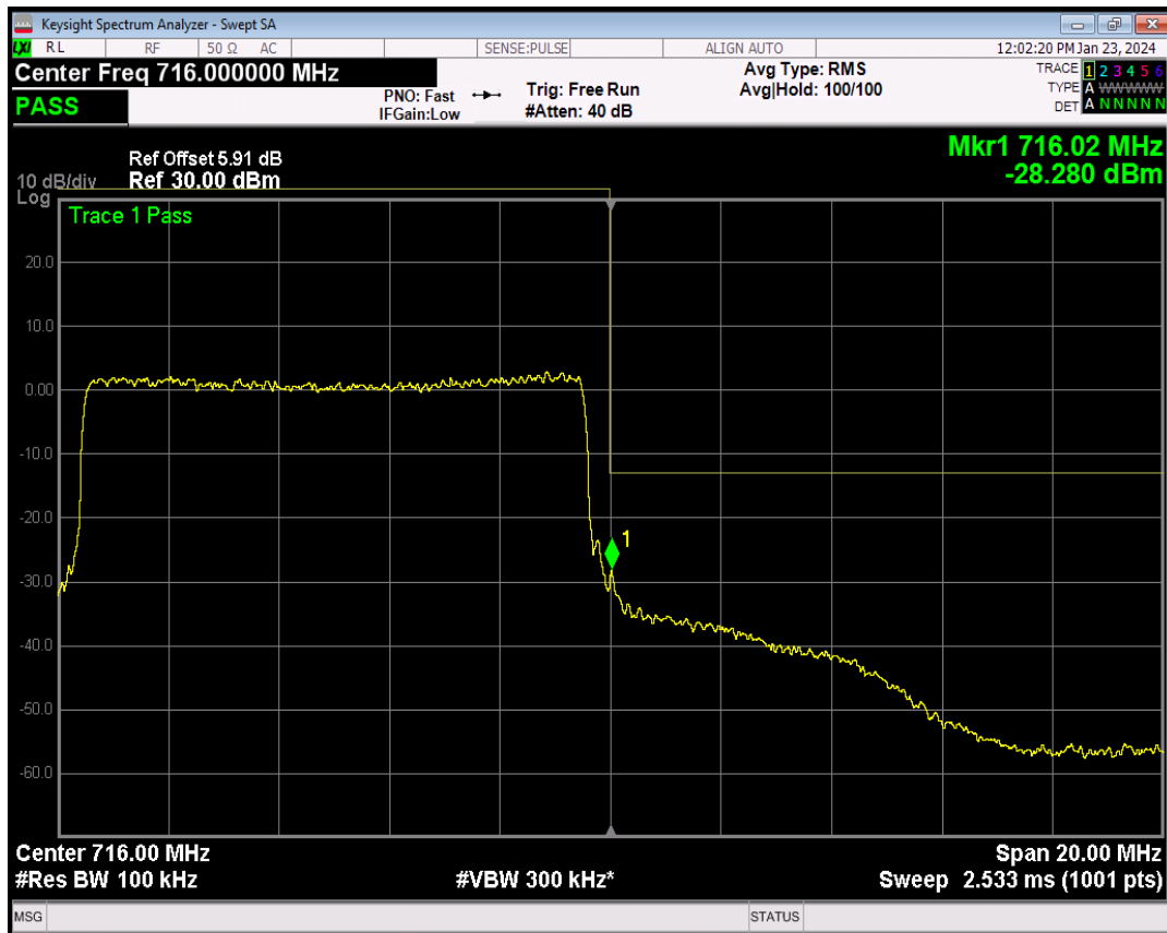
Band2 QPSK BW=1.4MHz Channel=18607 RB Size=1 Position=#0
