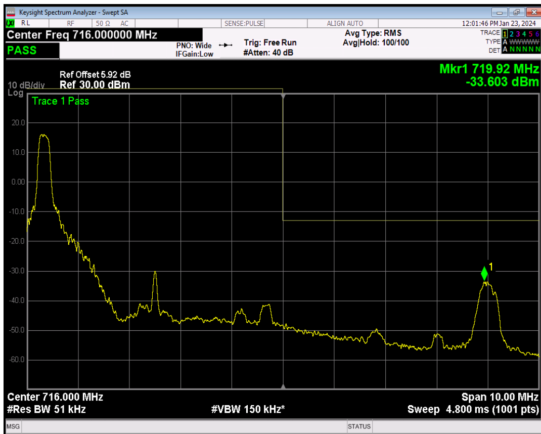
Band17 16QAM BW=5MHz Channel=23825 RB Size=1 Position=#Max
