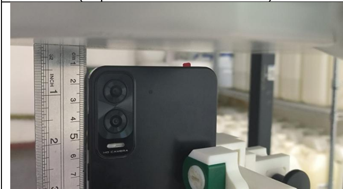
Top Side (Separation distance of 10mm)
