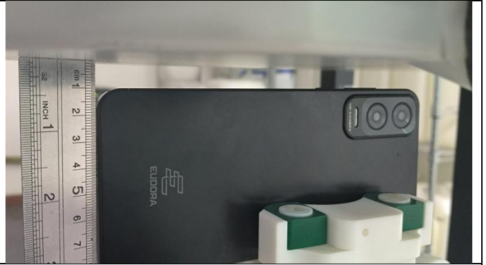
Bottom Side (Separation distance of 10mm)
