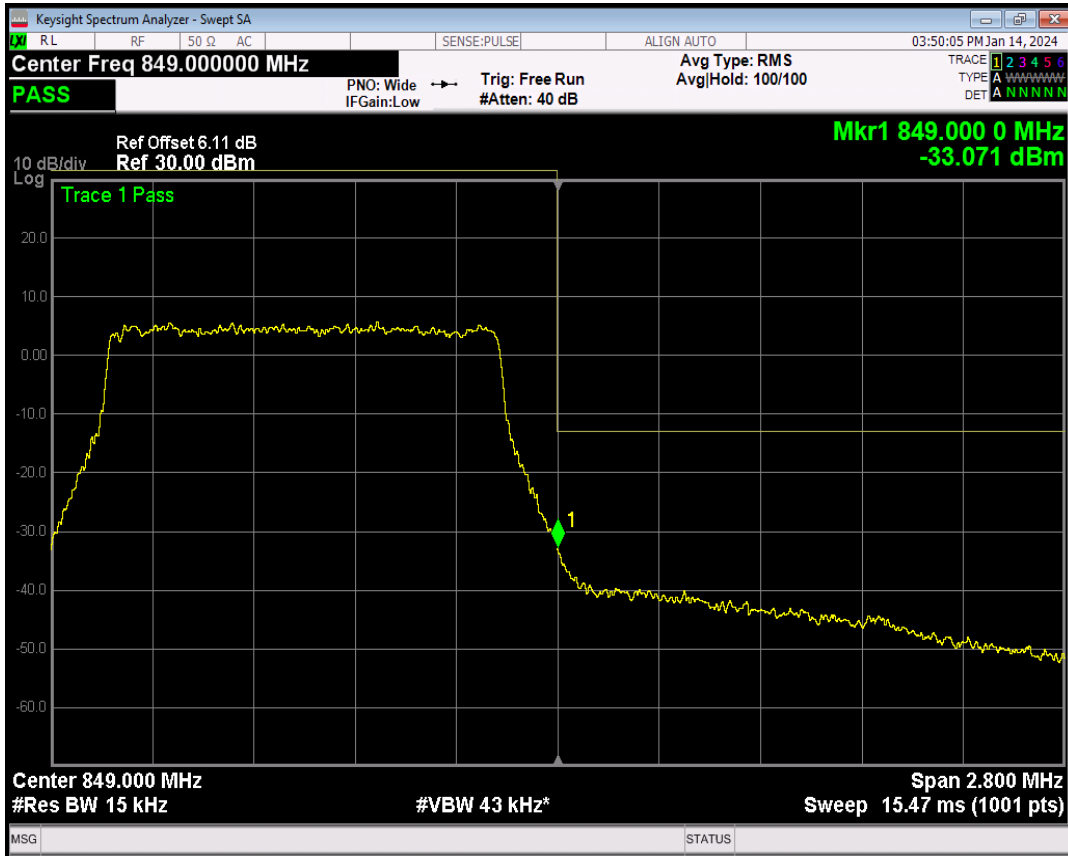
Band5 16QAM BW=1.4MHz Channel=20643 RB Size=1 Position=#0
