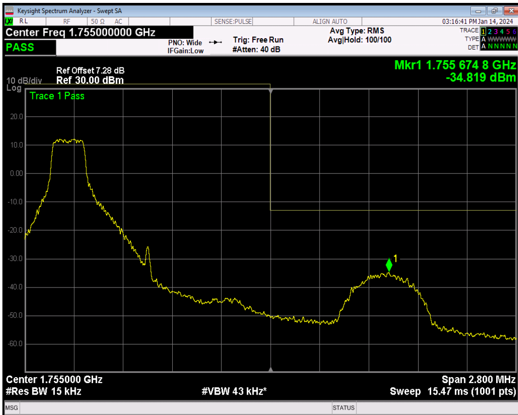
Band4 16QAM BW=1.4MHz Channel=20393 RB Size=1 Position=#Max
