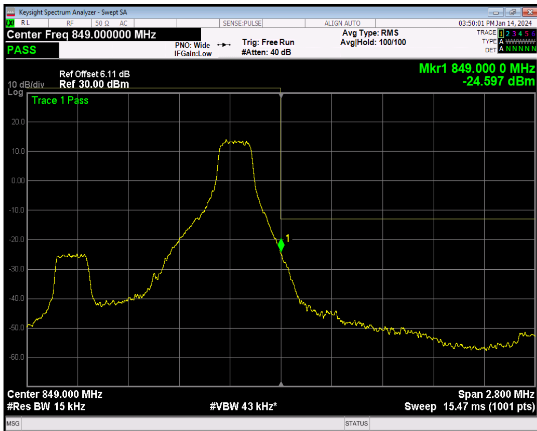
Band5 QPSK BW=1.4MHz Channel=20643 RB Size=6 Position=#0
