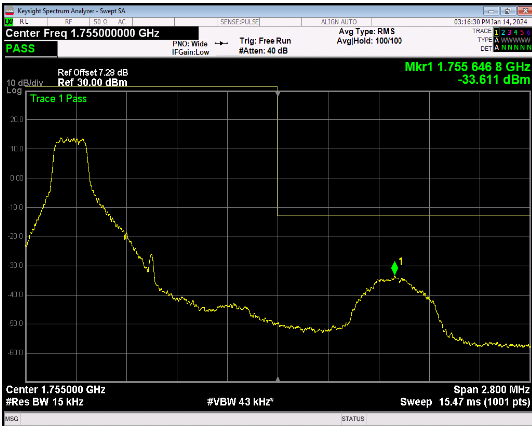
Band4 QPSK BW=1.4MHz Channel=20393 RB Size=6 Position=#0
