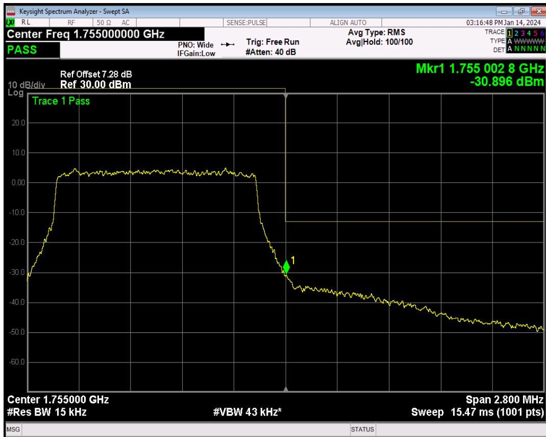
Band4 QPSK BW=3MHz Channel=19965 RB Size=1 Position=#0
