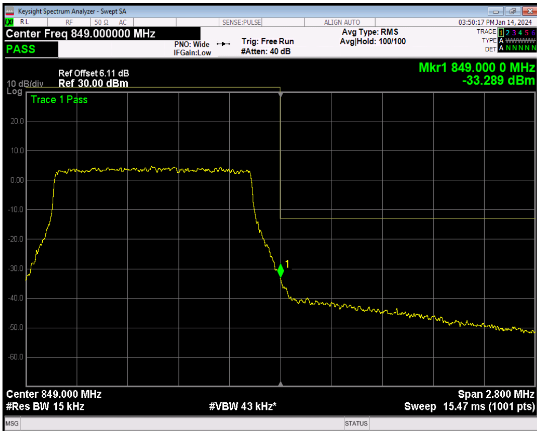
Band5 QPSK BW=3MHz Channel=20415 RB Size=1 Position=#0
