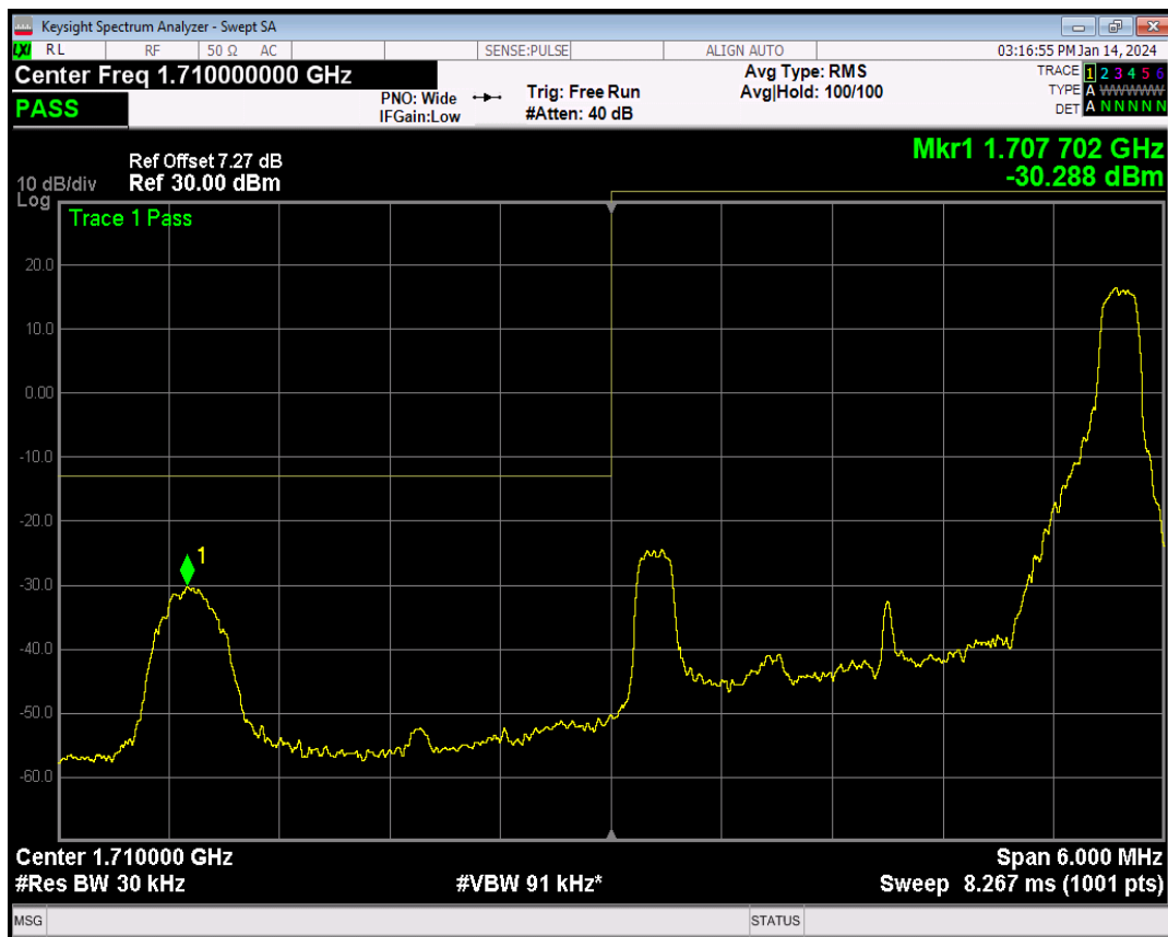
Band4 QPSK BW=3MHz Channel=19965 RB Size=15 Position=#0
