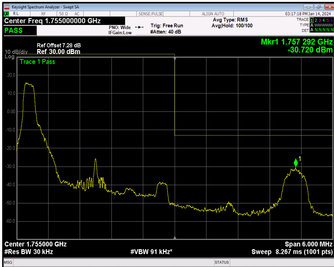
Band4 16QAM BW=3MHz Channel=20385 RB Size=15 Position=#0
