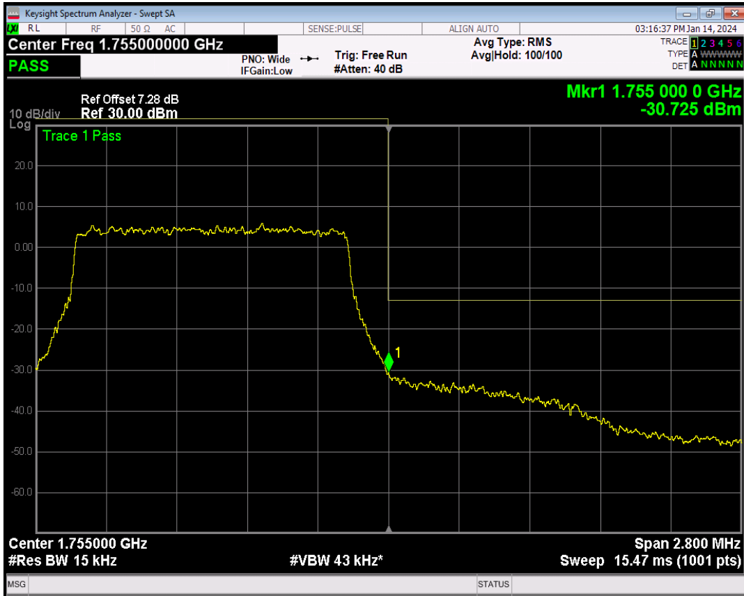
Band4 16QAM BW=1.4MHz Channel=20393 RB Size=1 Position=#0
