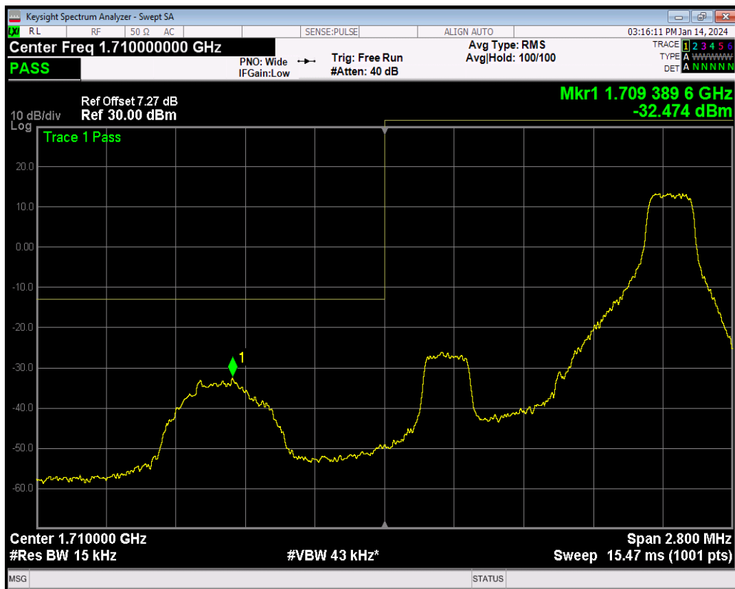
Band4 QPSK BW=1.4MHz Channel=19957 RB Size=6 Position=#0
