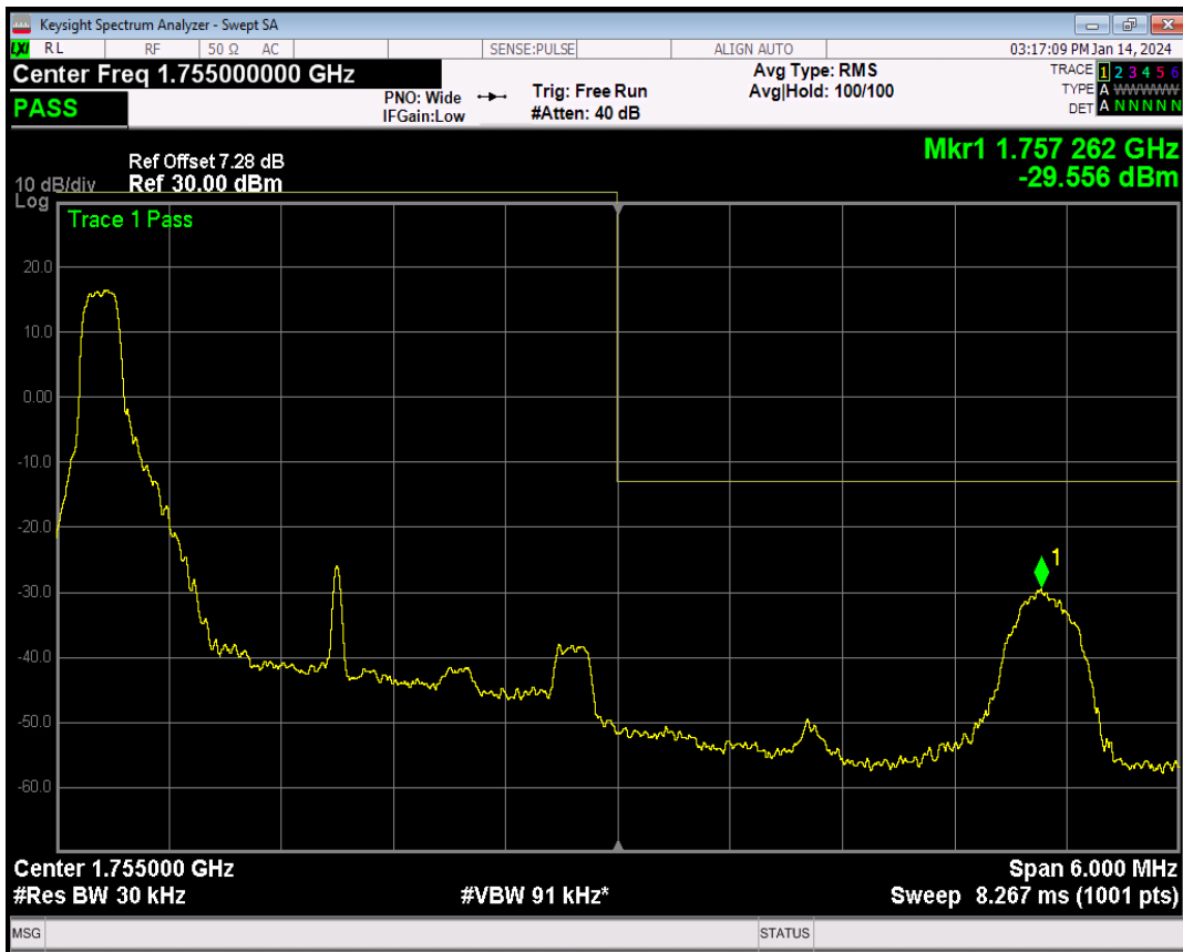
Band4 QPSK BW=3MHz Channel=20385 RB Size=1 Position=#Max
