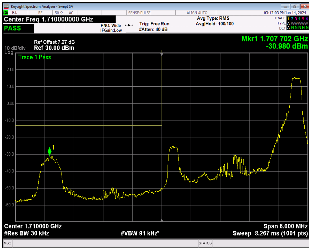
Band4 16QAM BW=3MHz Channel=19965 RB Size=15 Position=#0
