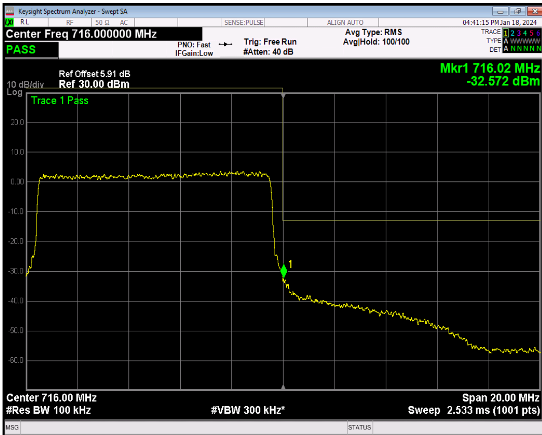
Band2 QPSK BW=1.4MHz Channel=18607 RB Size=1 Position=#0
