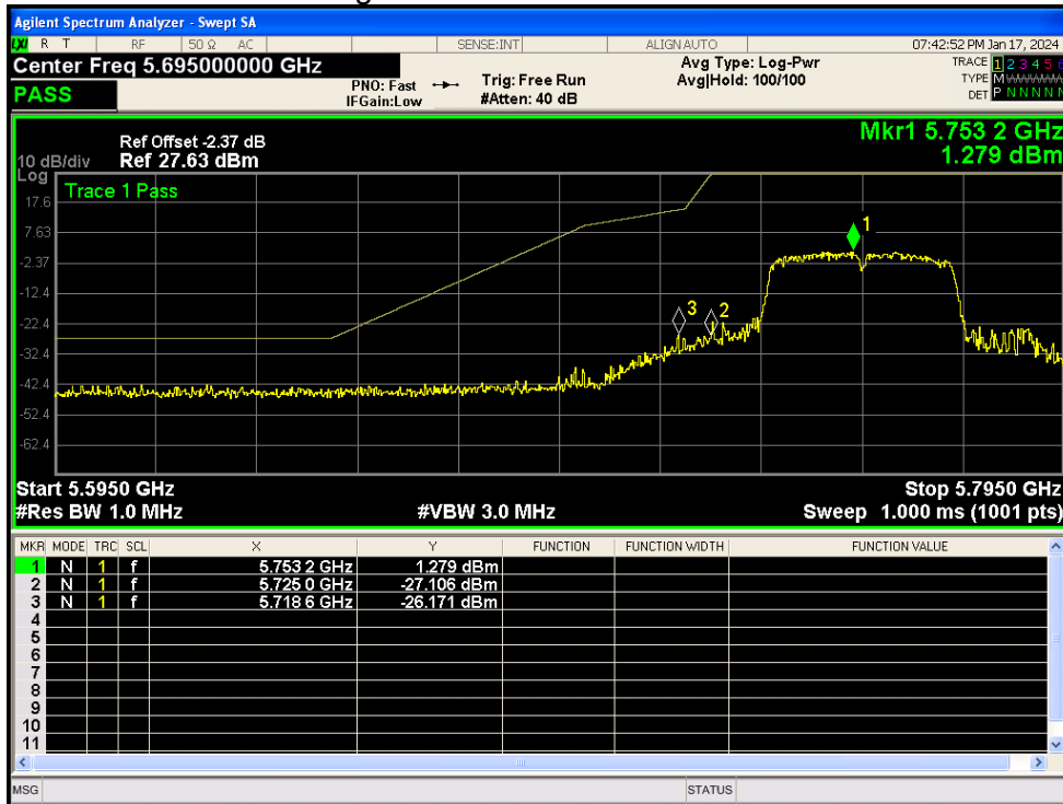
Band Edge NVNT ac40 5795MHz High Ant1
