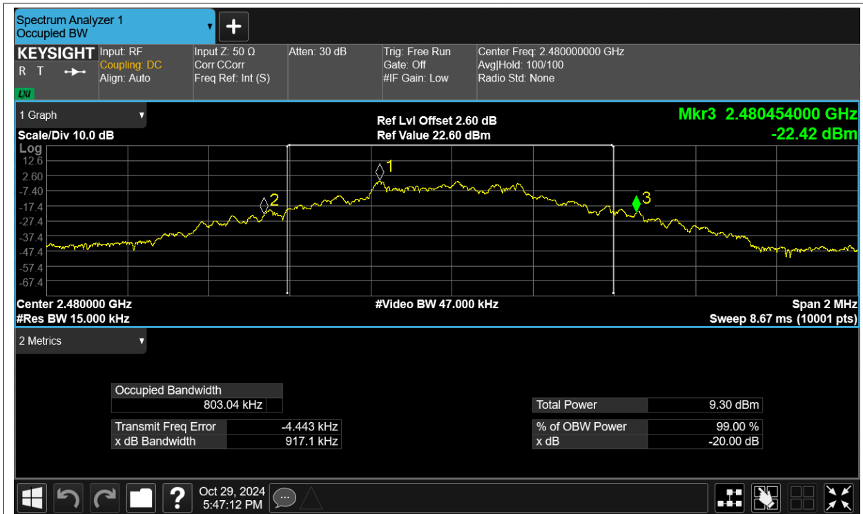
-20dB Bandwidth NVNT 2-DH1 2402MHz Ant1
