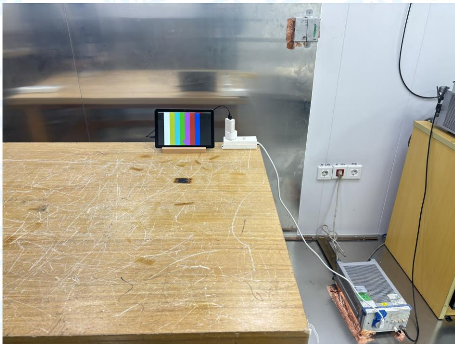
Photo of Setup for Conducted Emission
