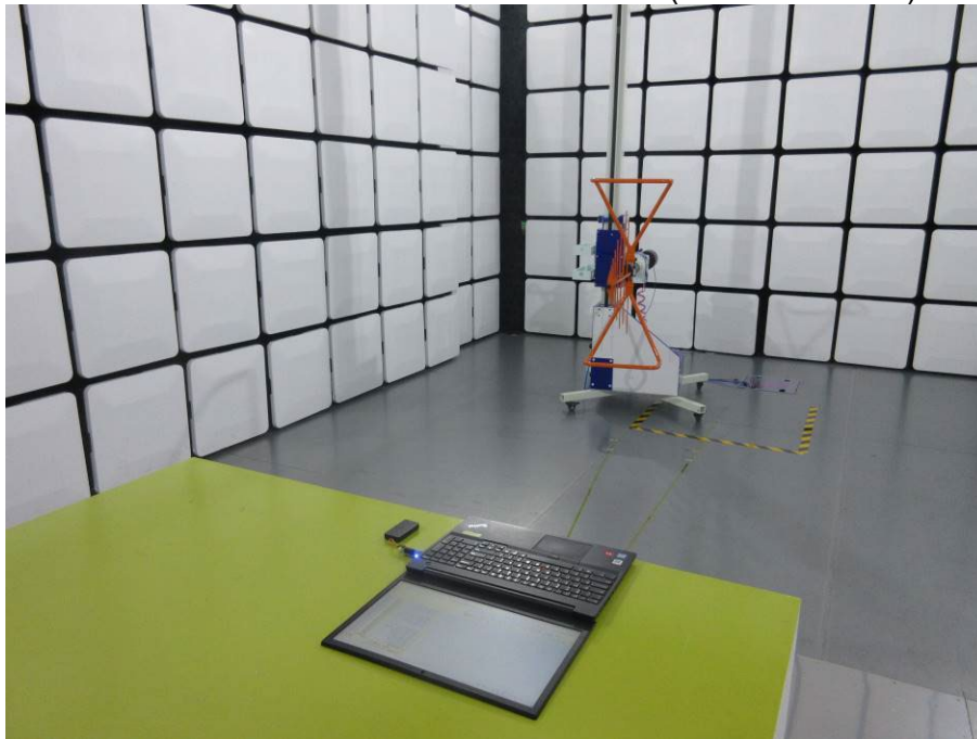
RADIATED RF MEASUREMENT SETUP (30MHz ~ 1 GHz)
