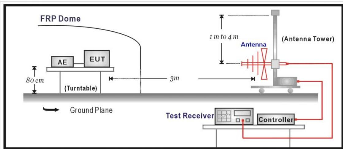
1GHz -40GHz Test Setup:
