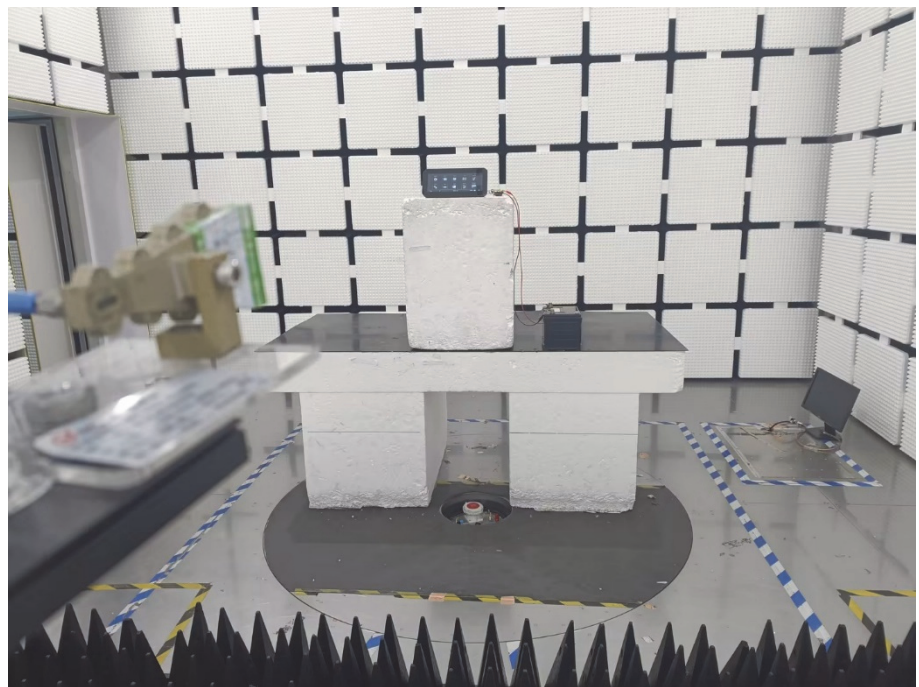
Radiation Emission Test Setup (Above 18GHz)
