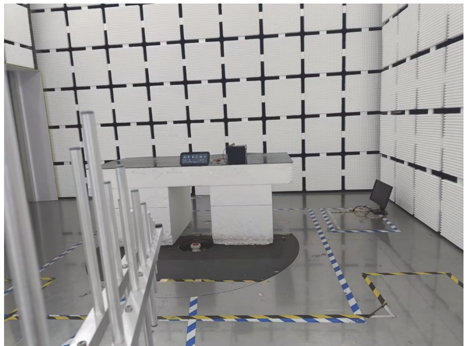
Radiation Emission Test Setup (30MHz to 1GHz)
