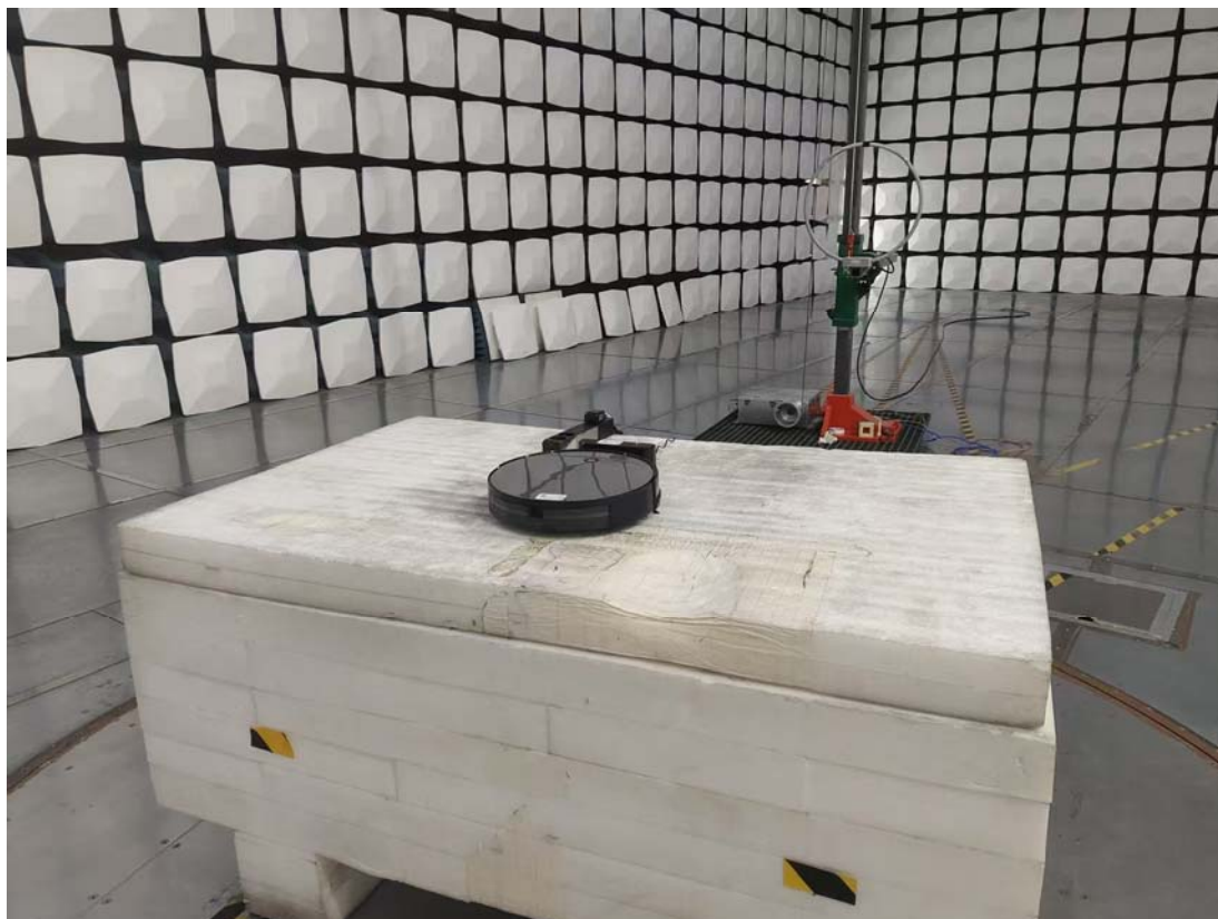
Radiated Emission 9k-30MHz Perpendicular View
