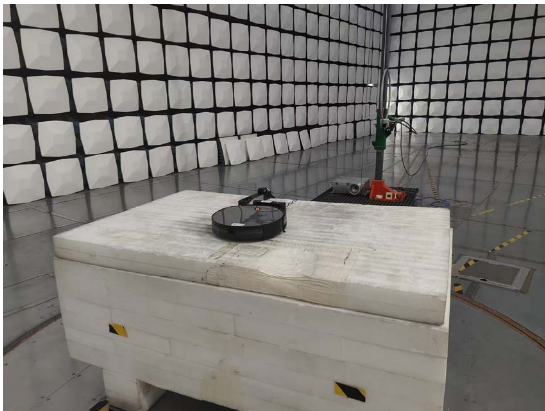
Radiated Emission 9k-30MHz Perpendicular View
