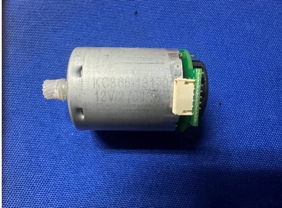
Details of: Motor for vacuum cleaning function (FBL6020-01F)
