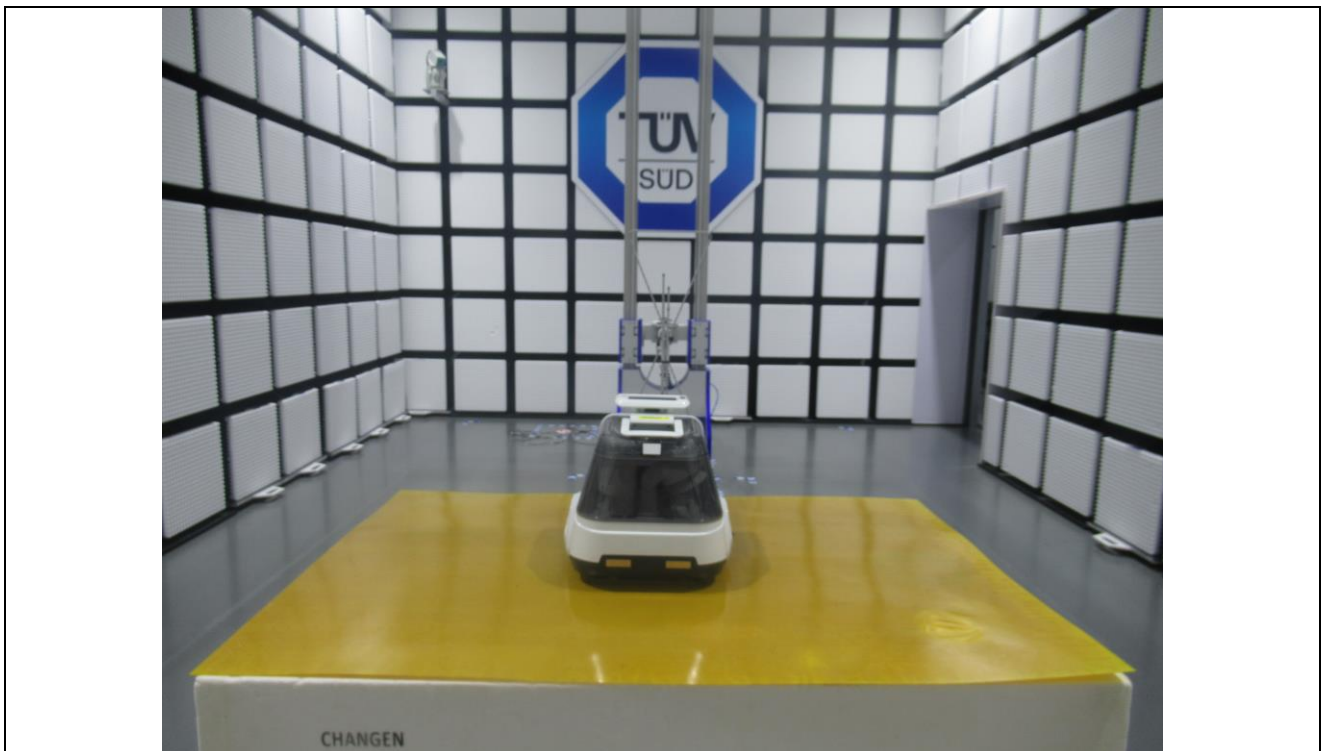
Radiated Emission test (30MHz to 1000MHz)
