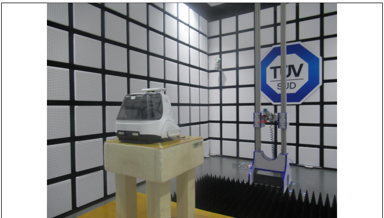
Radiated Emission test (1000MHz to 18000MHz)
