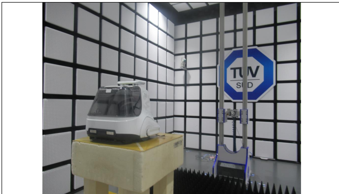
Radiated Emission test (Above 18000MHz)
