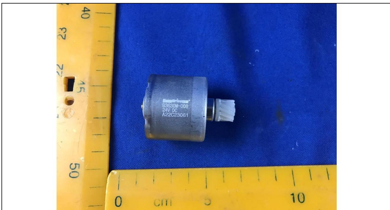
Details of: Motor for rolling brush (B4260M-025)
