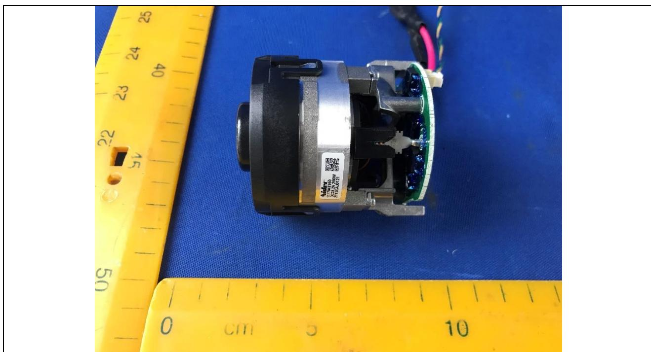
Details of: Motor for driving wheel (B2430M-020)
