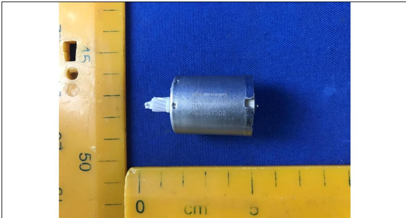
Details of: Motor for rotary brush (B3630M-008)
