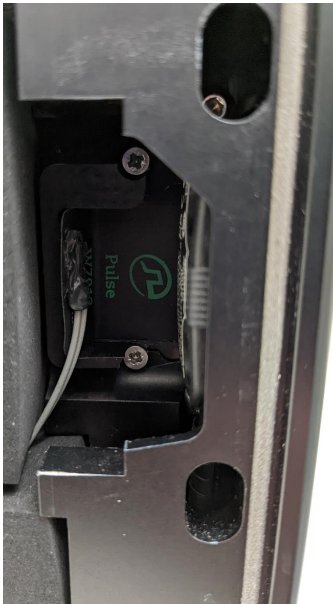
10000-1001 Highway1 NFC Antenna location in instrument
