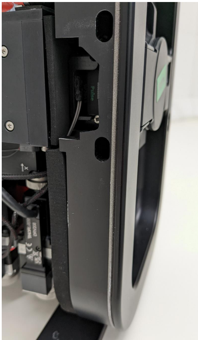
10000-1001 Highway1 NFC Antenna location in instrument
