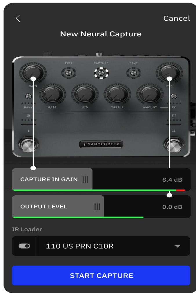
Ensure the target device's settings are set to your liking and the Nano Cortex's GAIN knob is at the minimum position.
