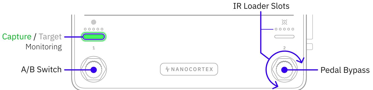
Press **Footswitch I** to toggle between the **Neural Capture** and the **Target Device**.
