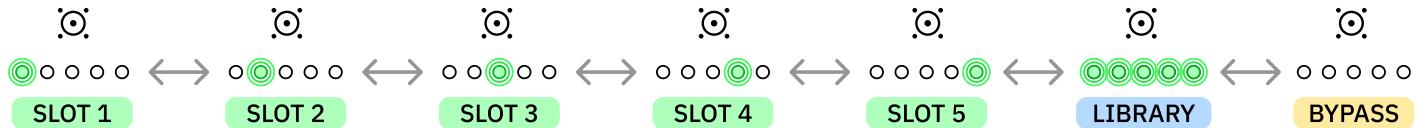
Turn **Footswitch II** clockwise or counterclockwise to navigate IR slots.
