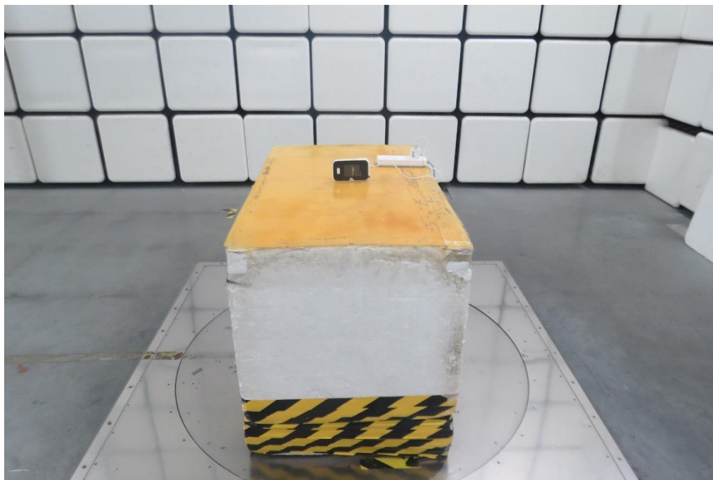
Picture 1 Radiated Emission Test Setup
