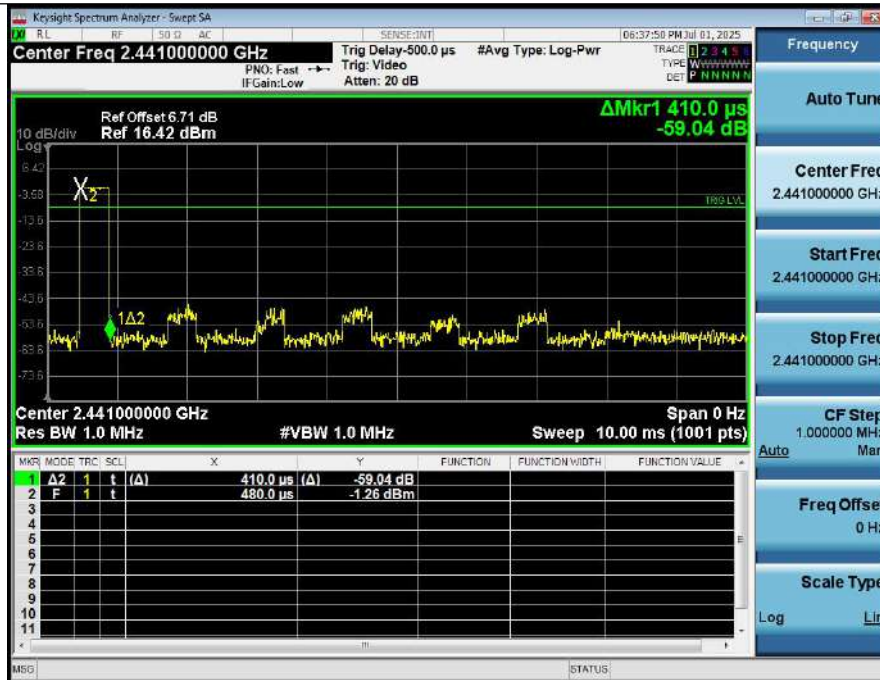
Dwell Time (Hopping) NVNT_ANT1_2-DH1_2441_00_Accumulated
