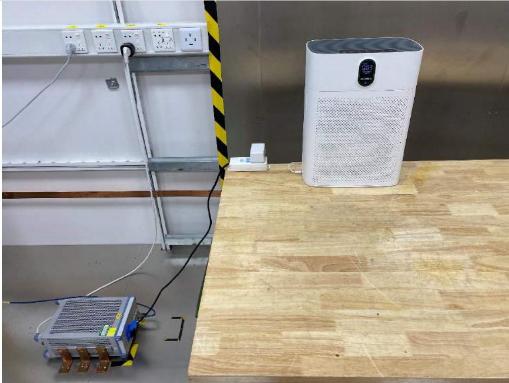
AC Power Line Conducted Emission
