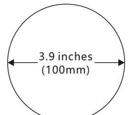
A, Drill 3.9-inch (100mm) diameter holes into the table top using a drill.
