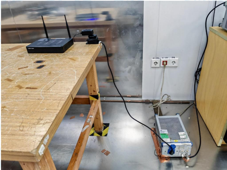
Photo of Setup for Radiated Emission (30MHz~1GHz)
