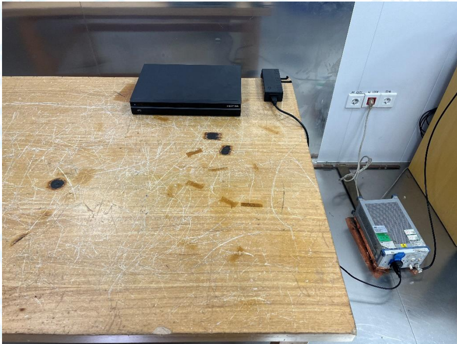
Photo of Setup for Radiated Emission (30MHz~1GHz)
