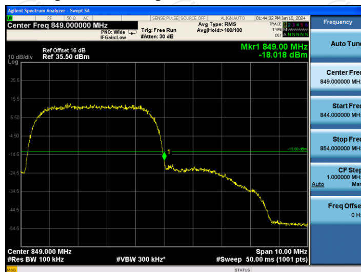
Higher Band Edge Plot on Channel 4233
