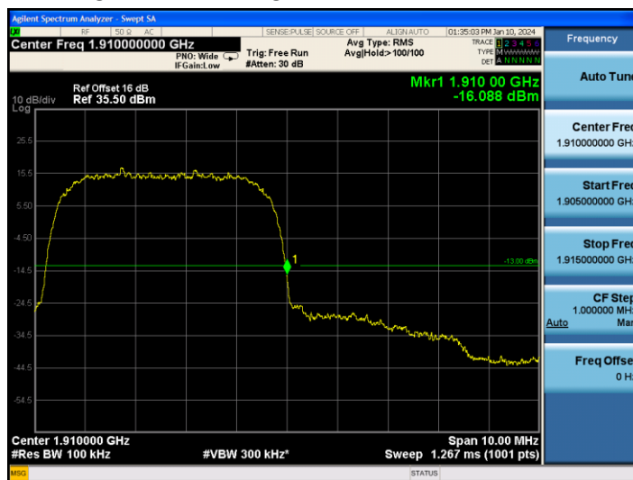
Higher Band Edge Plot on Channel 9538
