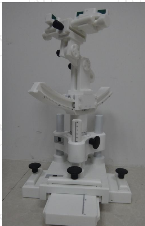
COMOSAR Mobile phone positioning system
