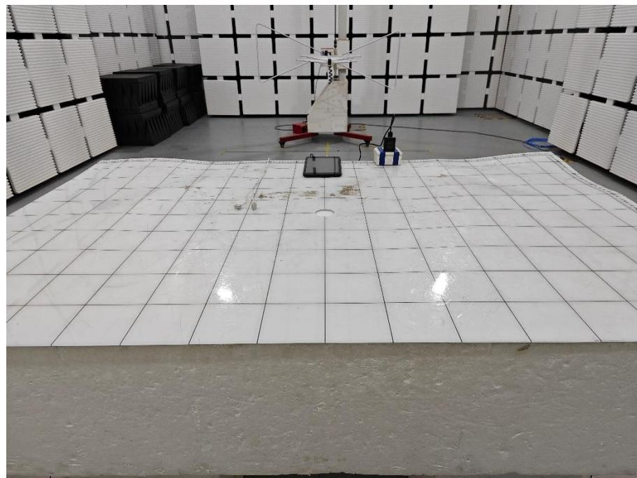
**Set-up for Radiated Emission (RE), Above 1GHz**
