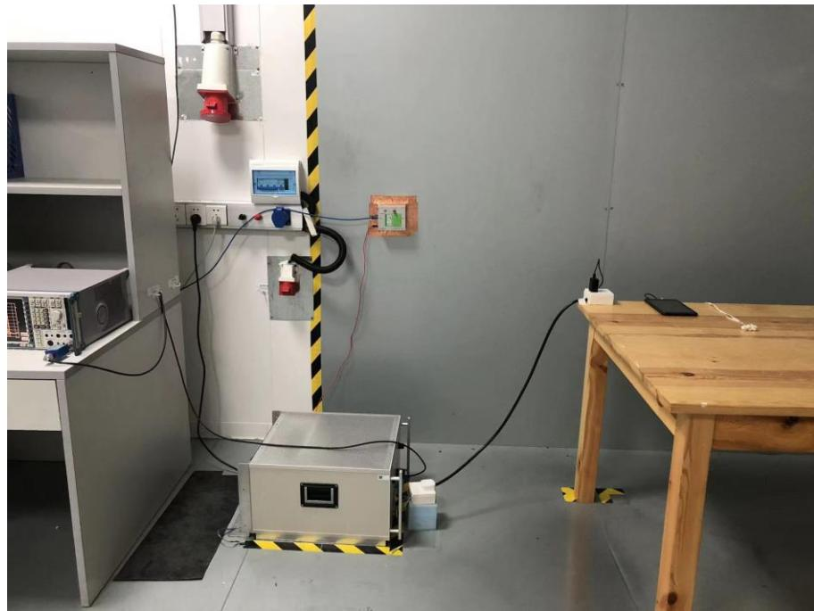
**Set-up for Radiated Emission (RE), Below 1GHz**
