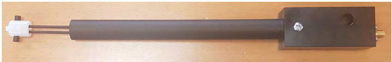
**Figure 1 – MVG COMOSAR Validation Dipole**
