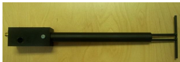
Figure 1 – MVG COMOSAR Validation Dipole
