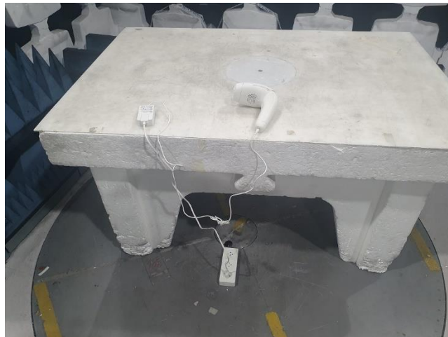
Picture 1 Radiated spurious emission test setup below 1GHZ.
