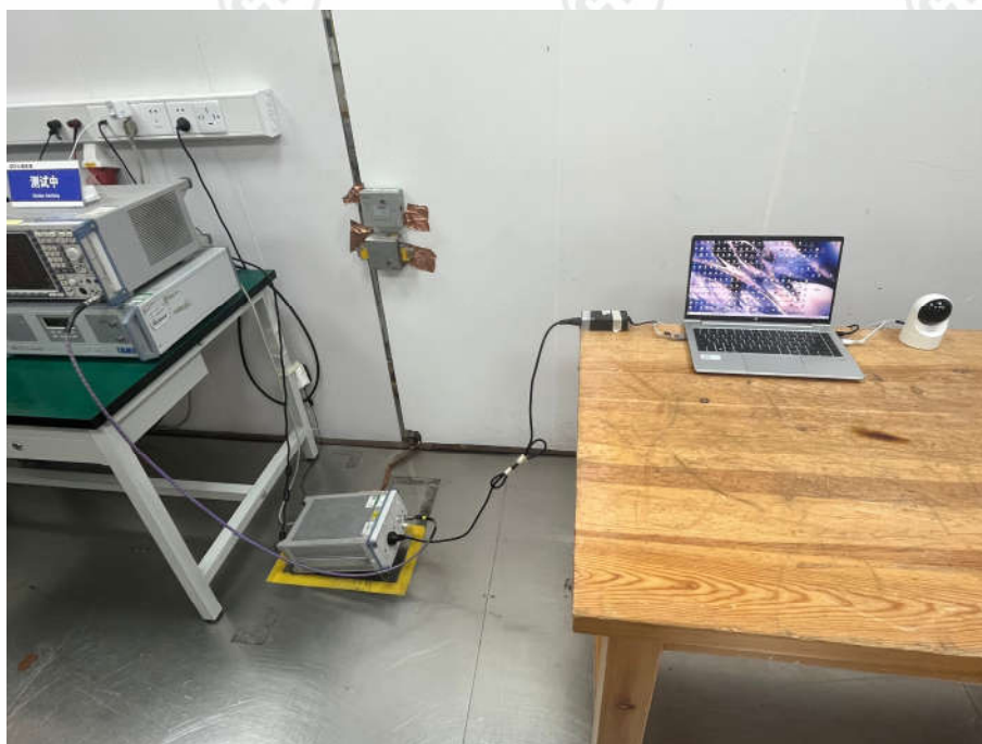
Conducted Emissions Test Setup
