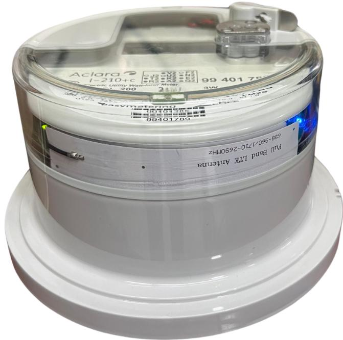
Verifying the correct operation of the smart meter i210 +C, record the necessary information and read the digital register, to complete the installation
