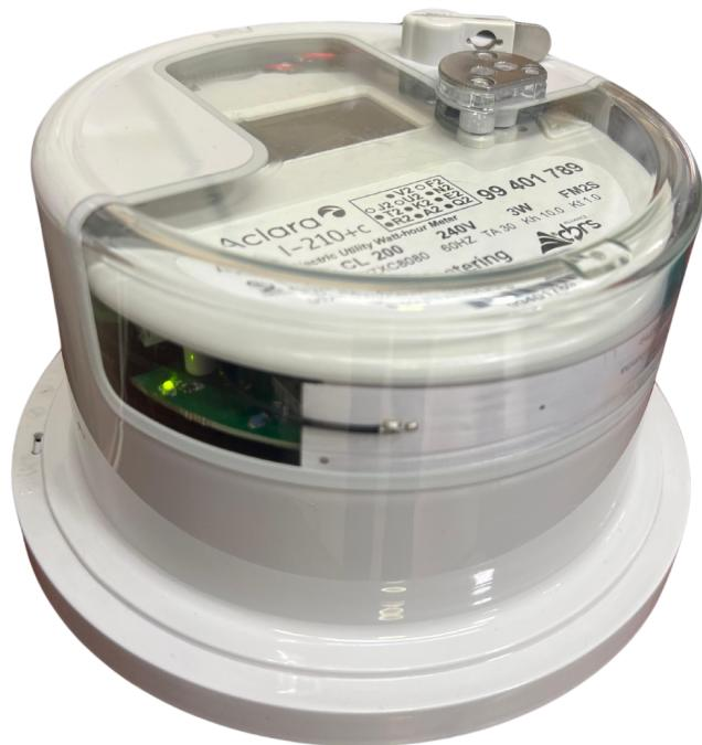
**Note** When the cellular module is turned on, the blue LED will light up and stay on, when it is attached to a cellular network, this LED will begin to blink.
