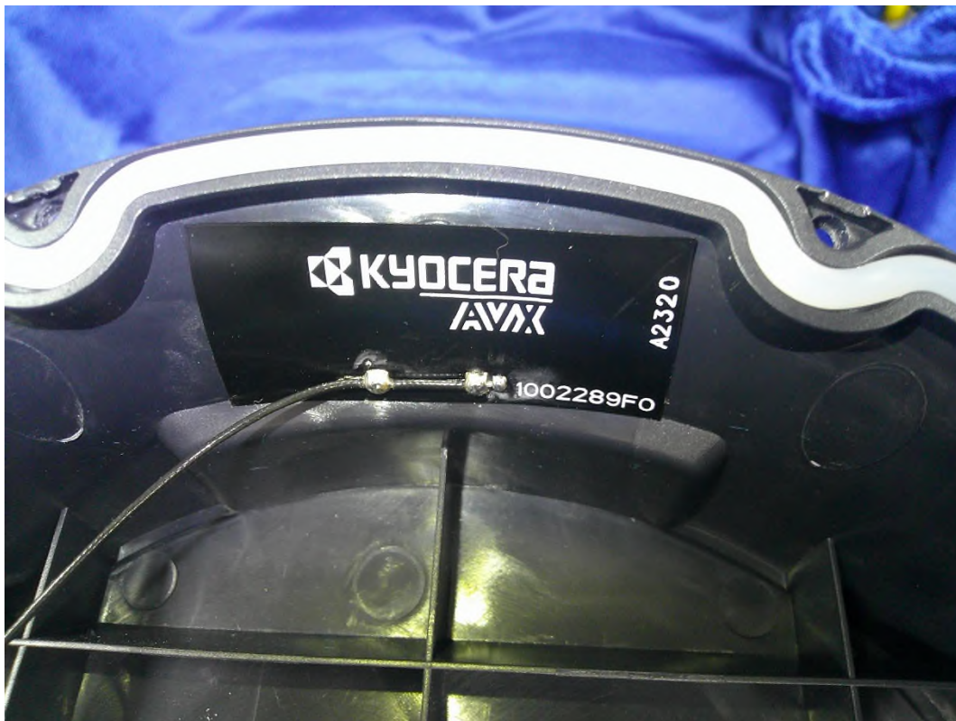
Photograph shows the location of the cellular antenna (Highlighted)
