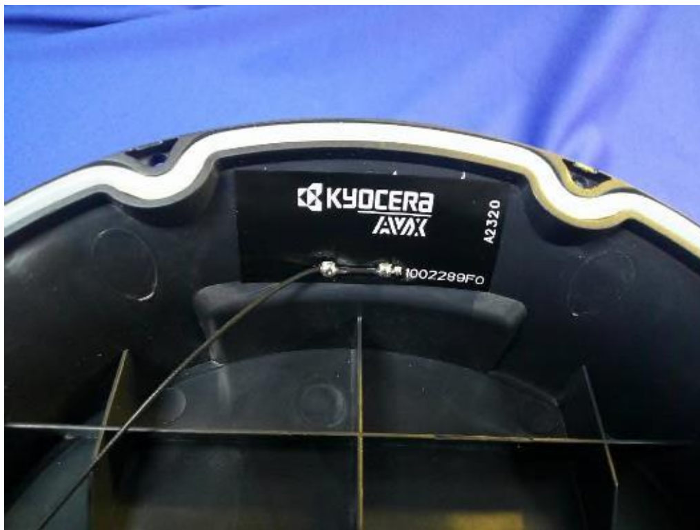
Photograph shows the EUTs cellular antenna
