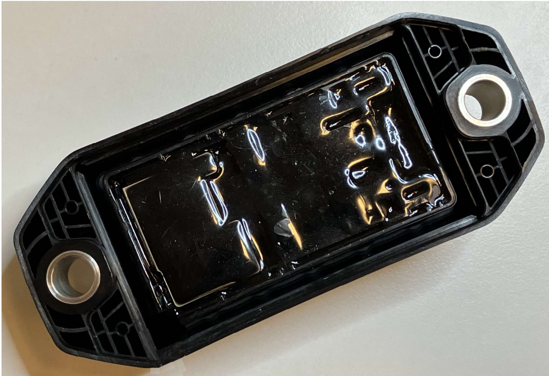
Inner box assembly with potting added
