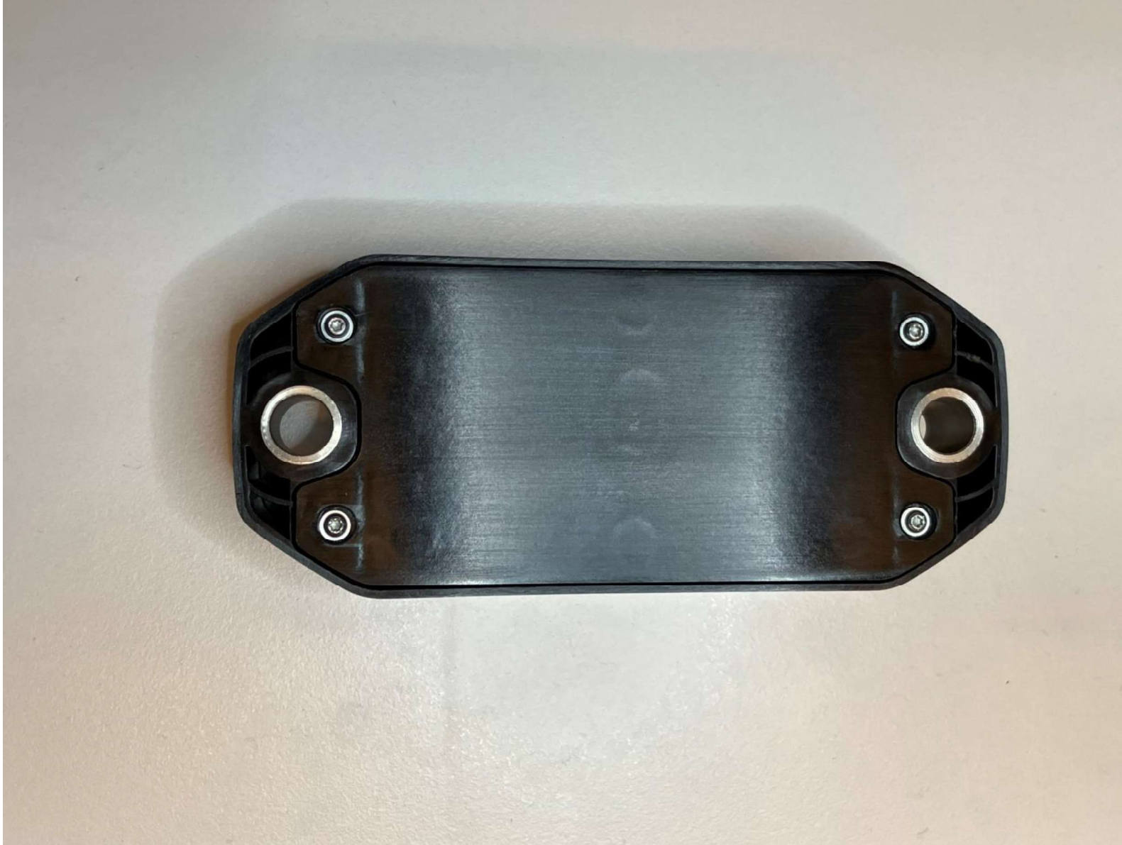
Bottom cover and four screws added
