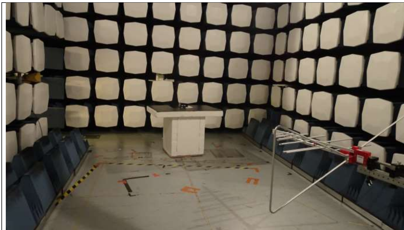
Picture 6, Radiated Spurious Emissions, common setup, TX 30 - 1000 MHz
