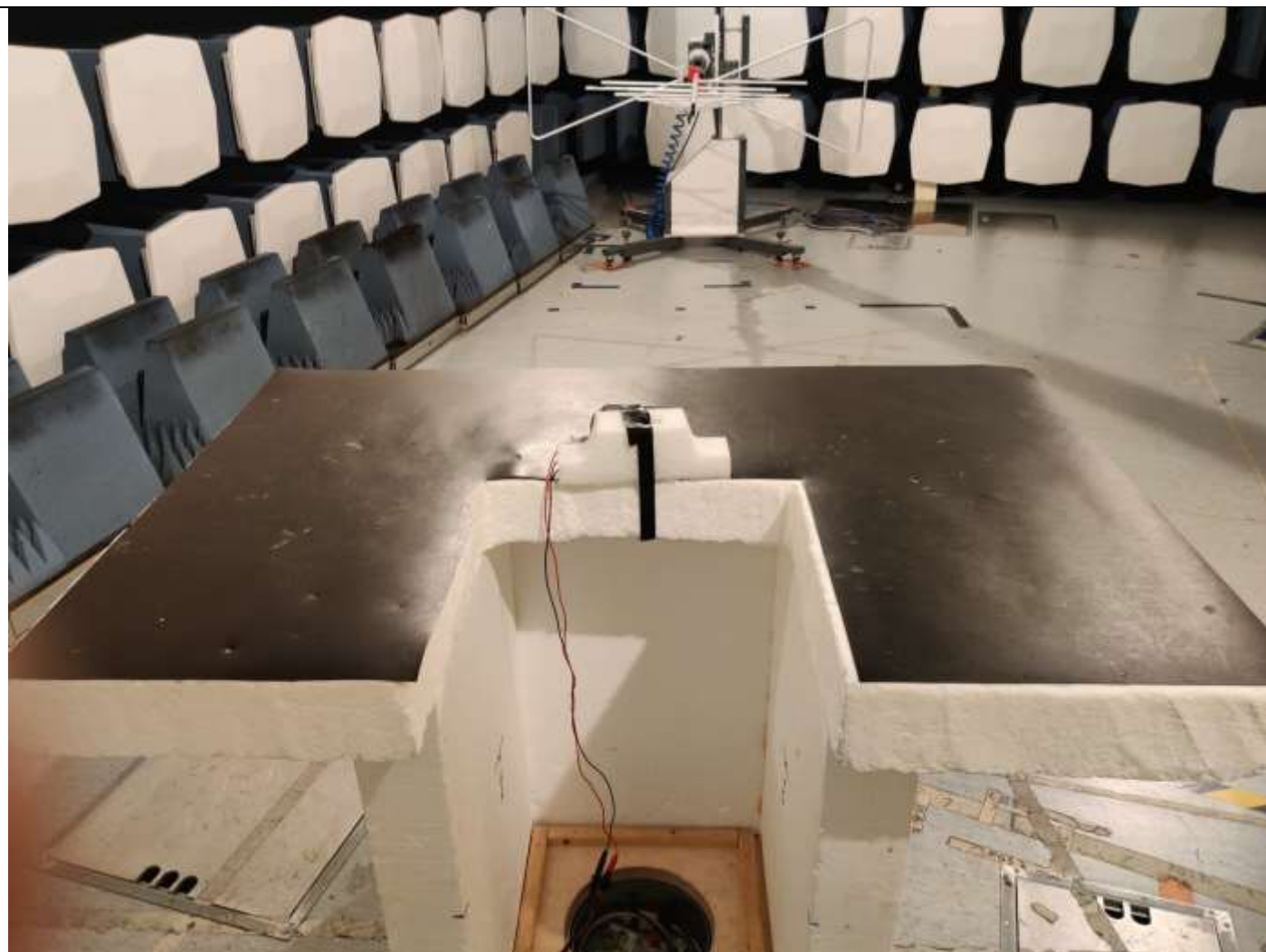
Picture 7, Radiated Spurious Emissions, back view, TX 30 - 1000 MHz
