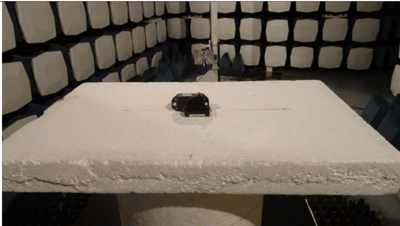
Picture 9, Radiated Spurious Emissions, EUT setup common
