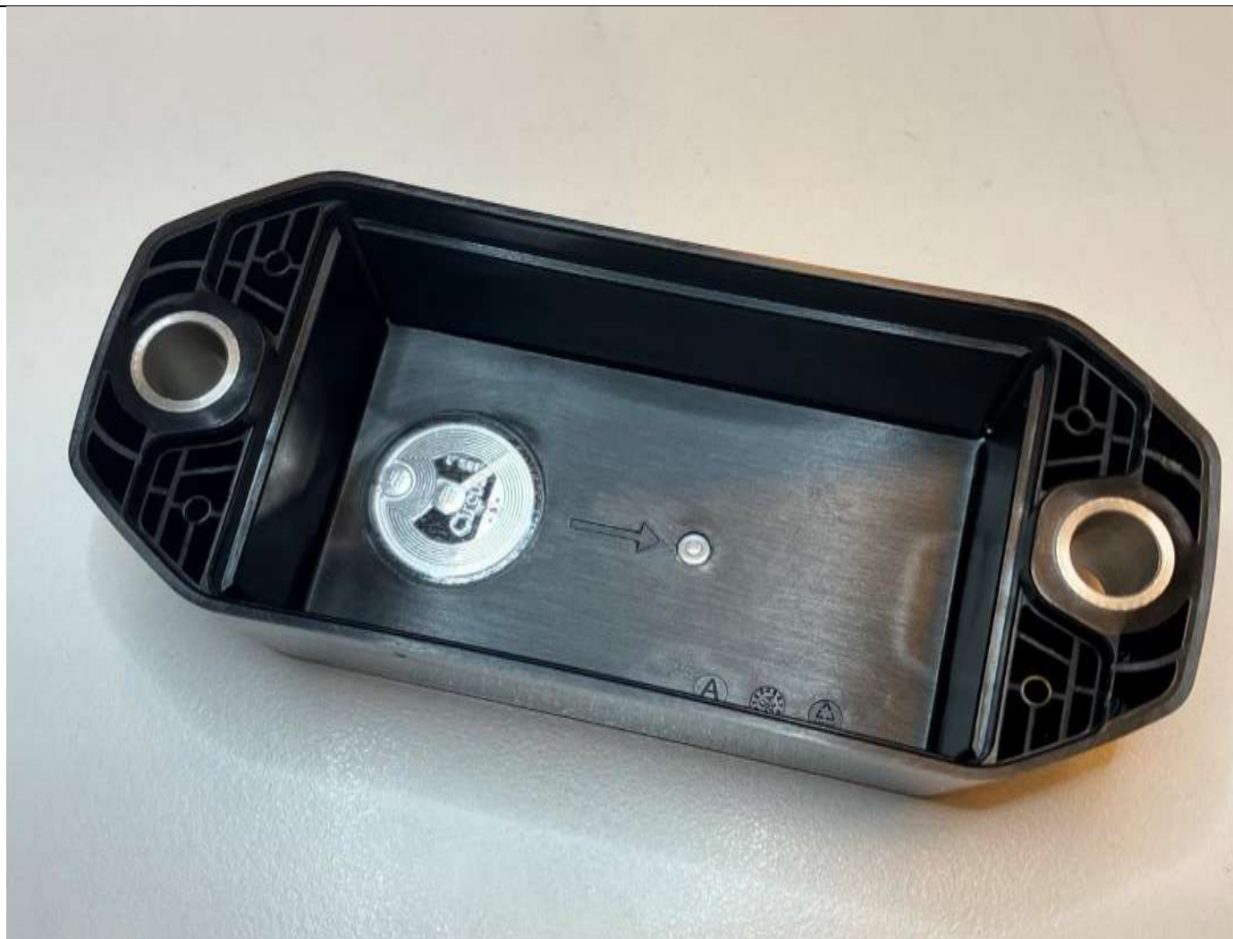
Picture 5, EUT A cover inside
