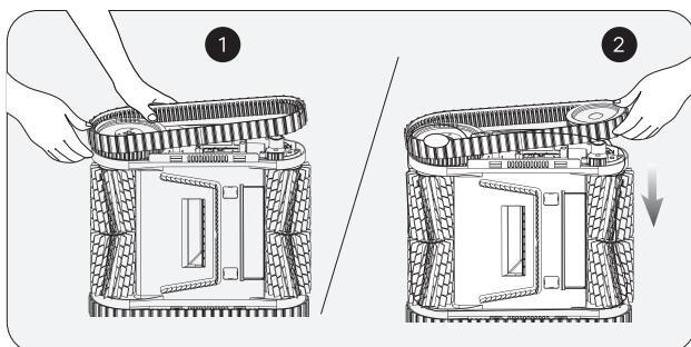
e. Re-install the guide sleeves by aligning their D-shaped openings with that of the shaft sleeves.
