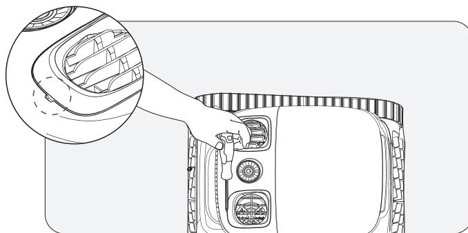
b. Remove the screws and drain cover.
