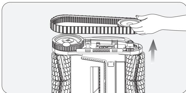
d. Align the gears on the new tracks with the gears on both wheels, then install the rear wheels and tracks together back onto the shaft sleeves.
