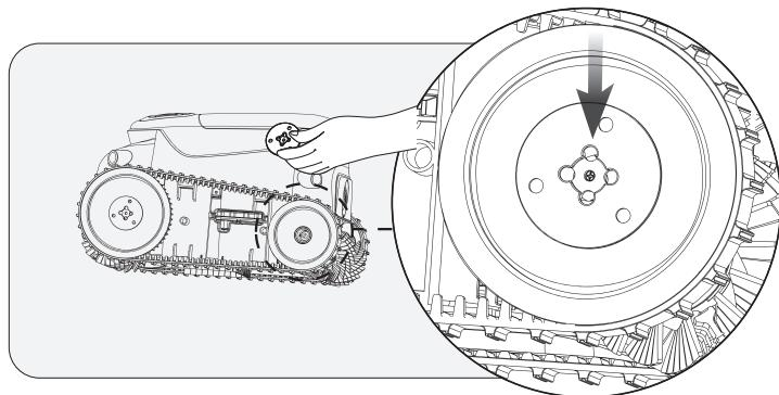
f. Tighten the screws and re-install the side cover plate.
