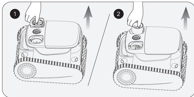
c. Remove any objects entangled in the drains fan blades, and then re-install the drain cover and screws.
