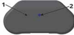
Fig. 3. SX Version - top view 1 - device enclosure; 2 - LED indicator
