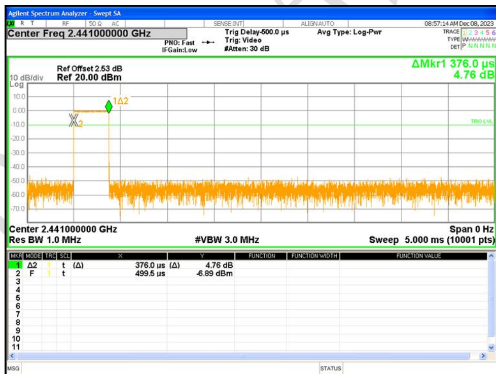
Dwell NVNT 1-DH1 2441MHz Ant1 One Burst
