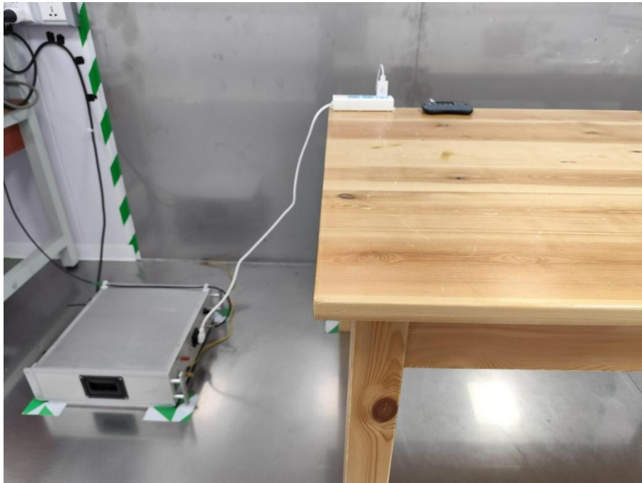
Conducted Emission at AC power line
