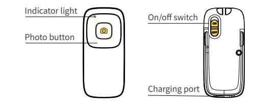
1. Toggle the switch (ON/OFF) on the back of the remote control, the remote control indicator light will flash automatically.
