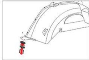
5. Run wiring for rear Rock Light along the pinch seam, securing with zip ties where necessary and up through the fender into the engine bay.
