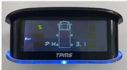
Long press the middle button for 3 seconds to enter the setting interface, short press the right button for 5 times, and display 5 in the upper left corner Set the rear wheel high voltage alarm value in this mode. Short press the middle button, the pressure value flashing state, press the left button to reduce, press the right button to add, press the middle button to confirm. Long press the right button to exit the setting mode.
