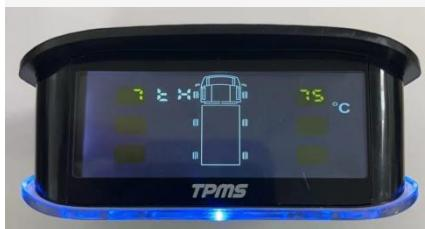
Long press the middle button for 3 seconds to enter the setting interface, short press the right button for 7 times, and display 7 in the upper left corner Temperature alarm value setting in this mode. Short press the middle button, the temperature value flash state, press the left button to reduce, press the right button to add, press the middle button to confirm. Long press the right button to exit the setting mode.
