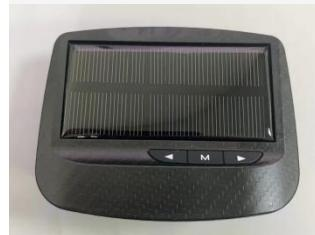
Long press the left button to switch the machine on and off
