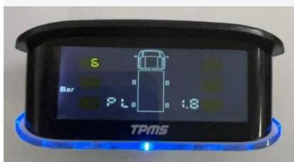
Long press the middle button for 3 seconds to enter the setting interface, short press the right button for 6 times, and display 6 in the upper left corner Set the alarm value setting the rear wheel in this mode. Short press the middle button, the pressure value flashing state, press the left button to reduce, press the right button to add, press the middle button to confirm. Long press the right button to exit the setting mode.
