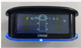
Long press the middle button for 3 seconds to enter the setting interface, short press the right button twice, the upper left corner shows 2, Change the temperature units in this mode. Short press the middle button, the temperature unit flash state, press the left button to switch, press the middle button to confirm. Long press the right button to exit the setting mode.
