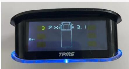
Long press the middle button for 3 seconds to enter the Settings interface, short press the right button for 3 times, and display 3 PH in the upper left corner
