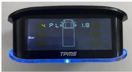
Long press the middle button for 3 seconds to enter the Settings interface, short press the right button for 4 times, and display 4 PL in the upper left corner
