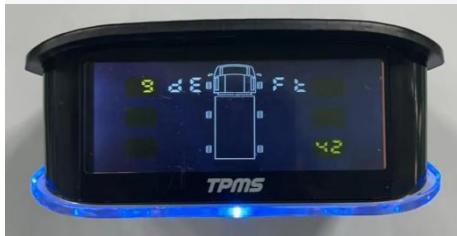
Long press the middle button for 3 seconds to enter the setting interface, short press the right button for 9 times, the upper left corner shows 9 to restore the factory setting in this mode, short press the middle button, display NO / YES
