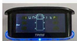
Long press the middle button for 3 seconds to enter the setting interface, short press the right button once, and display 1 in the upper left corner. Change the air pressure unit in this mode. Short press the middle button, the pressure unit flashing state, press the left button to switch, press the middle button to confirm. Long press the right button to exit the setting mode.
