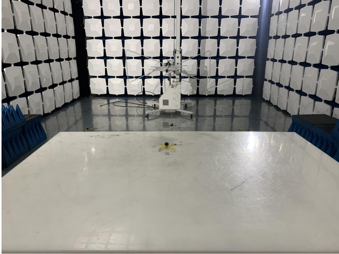
Above 1GHz for radiated emission test setup
