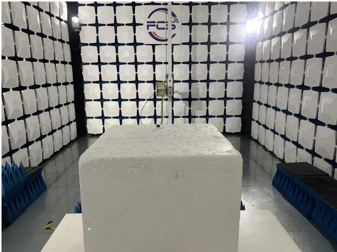
Above 1GHz for radiated emission test setup
