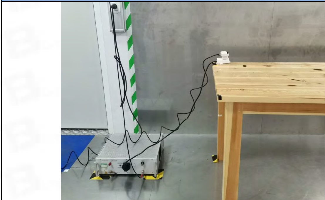
Conducted Emission at AC power line
