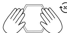
5. Identify the correct connecting port on the second light, snap the second light into place.
