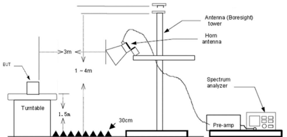
Above 18 GHz shall be extrapolated to the specified distance using an extrapolation factor of 20 dB/decade from 3m to 1m.
