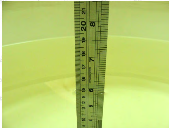
Photo of Liquid Height for Body SAR
