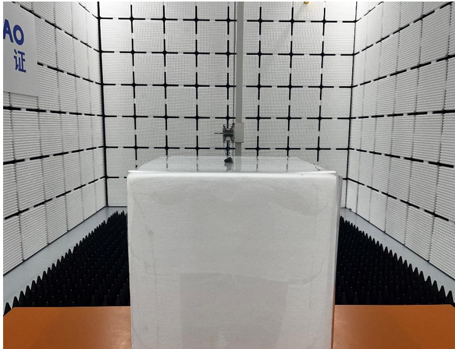
Radiated Emission Above 1GHz (Left ear)
