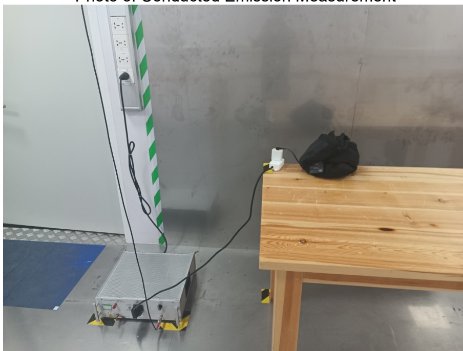
FCC ID: 2BCXN-F1117 Photo of Conducted Emission Measurement
